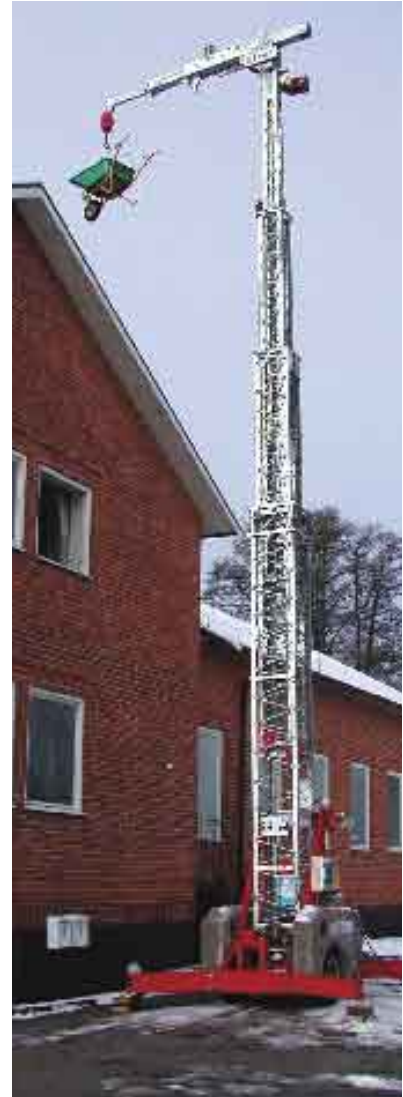
HAKI City C800 telescope crane is a flexible aid for lifts up to 800 kg. It can be erected, dismantled and moved in seconds.
