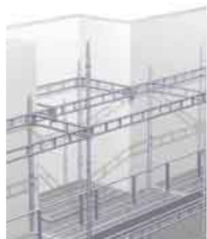
With beam riders you can add to the scaffolding virtually anywhere along the façade.
