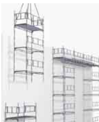
A great advantage is that you can erect whole sections on the ground and then lift them into position. This could save a lot of time when erecting the scaffolding, and especially when moving whole sections to other areas within the site.
